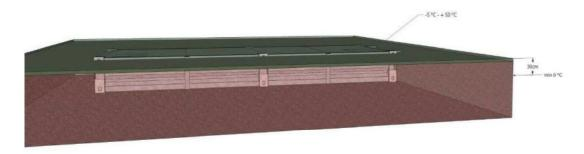
The use with temperature below  $0^{\circ}$ C is possible, if the surrounding soil does not freeze to depth of more than 30 cm. The use with lower temperature is possible only with additional thermal insulation, heating or by digging it deeper and it is always solved individually.
